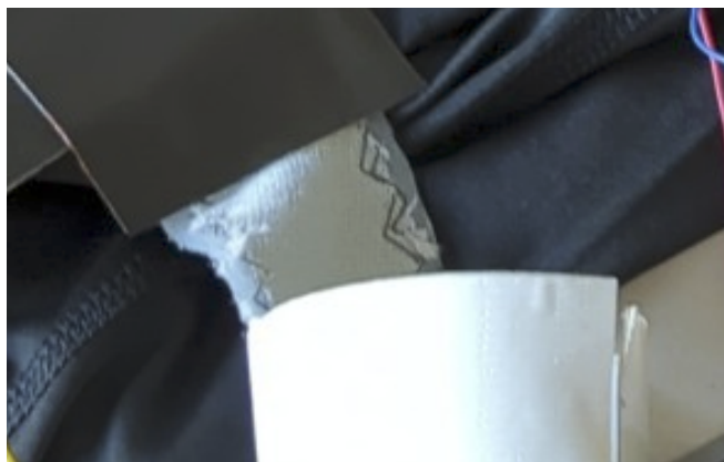
Figure 2: Capacitance sensor integrated into the shirt
