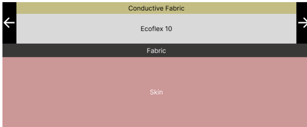
Figure 1: Diagram of the sensor design
